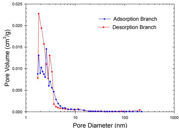
Figure 10. Pore Size Distributions for 6A.
