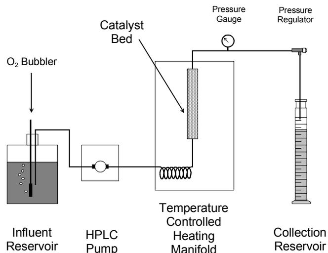
**Figure 4.** Catalyst Evaluation Test Stand.
