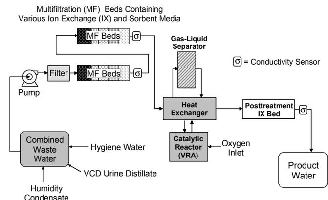
**Figure 1.** International Space Station Water Processor Assembly (WPA) Schematic.
