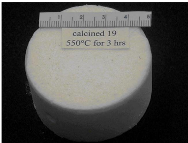
**Figure 3.** Calcined MCF Monolith (scale in cm).
