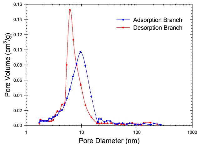
Figure 8. Pore Size Distributions for 1C.
