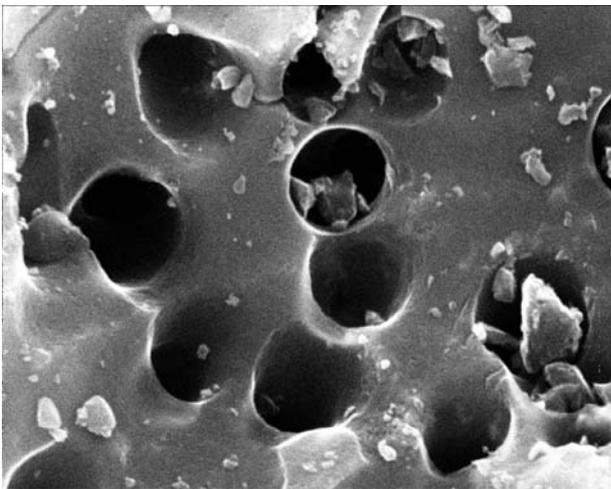
FIGURE 2 Scanning electron micrographs of Barnebey-Sutcliffe 580-26 activated carbon. Top X2,000, Bottom X 10,000 magnification
