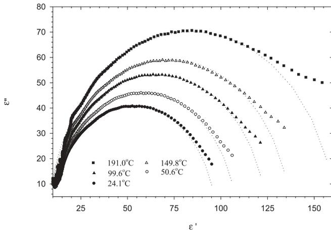
FIGURE 6 Cole–Cole plot for coconut shell activated carbon
