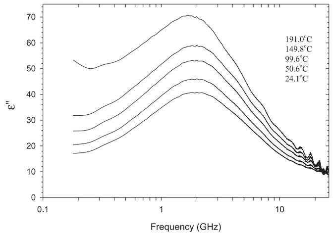
FIGURE 4 Imaginary component of complex permittivity vs. frequency and temperature
