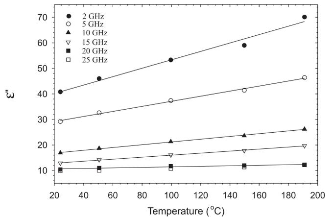
FIGURE 5 Dielectric loss versus temperature for a range of microwave frequencies
