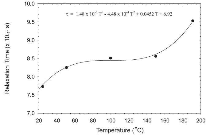
FIGURE 7 Polarization relaxation time versus temperature
