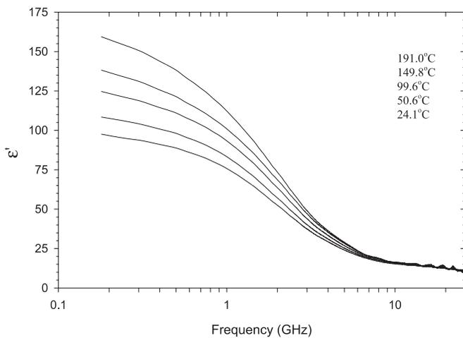
FIGURE 3 Real component of complex permittivity vs. frequency and temperature
