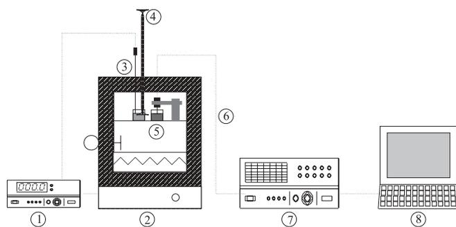
**FIGURE 1** Complex permittivity test apparatus: 1) temperature controller, 2) oven, 3) thermocouple, 4) Hg thermometer, 5) coaxial dielectric probe immersed in sample, 6) high temperature semi-rigid coaxial cable, 7) vector network analyzer, and 8) computer
