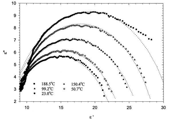
Fig. 5. Cole–Cole plot for Alltech 5769 coconut shell activated carbon.
