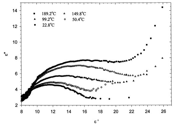
Fig. 7. Cole–Cole plot for Sigma C-3014 kilned peat activated carbon.
