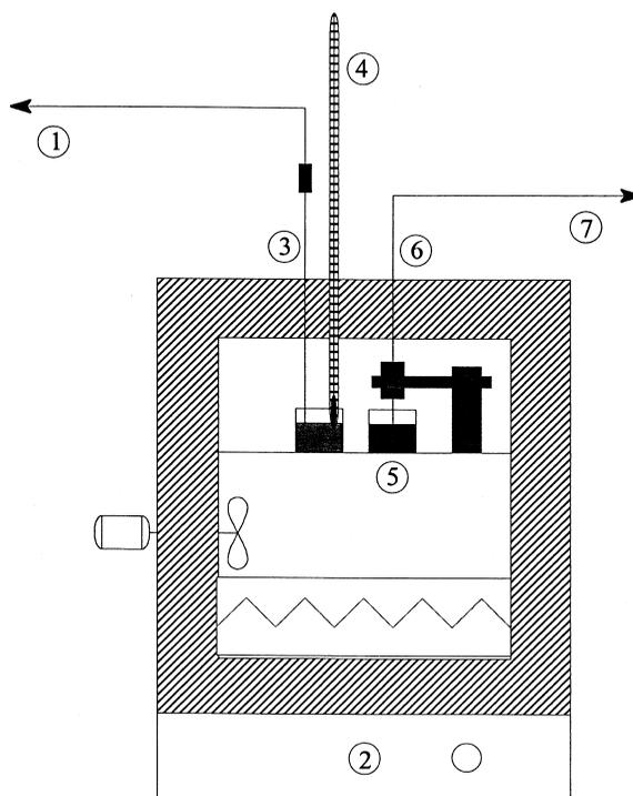
Fig. 1. Complex permittivity test apparatus: (1) temperature controller, (2) oven, (3) thermocouple, (4) Hg thermometer, (5) coaxial dielectric probe immersed in sample, (6) high-temperature semi-rigid coaxial cable, (7) vector network analyzer, and computer.
