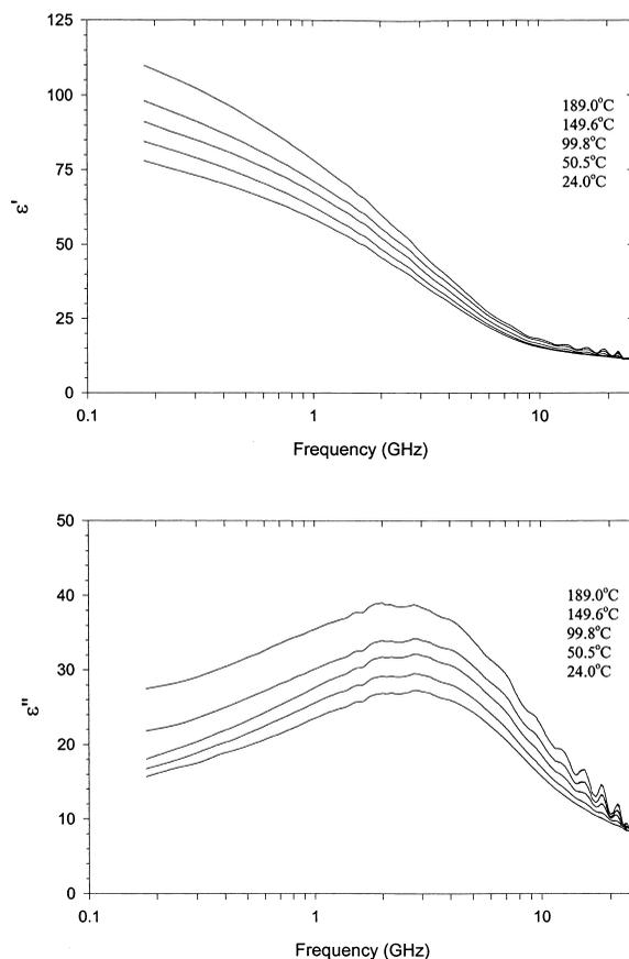
Fig. 2. Complex permittivities of Calgon APA bituminous activated carbon.
