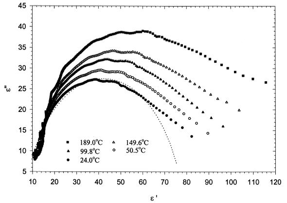
Fig. 6. Cole–Cole plot for Calgon APA bituminous activated carbon.
