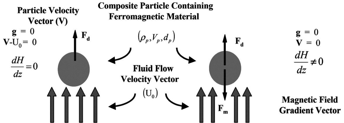
Fig. 2. Balance of forces acting on a fluidized particle containing ferromagnetic material in, a) a fluidized bed in microgravity in the absence of a magnetic field, and b) a gradient-magnetically assisted stabilized bed in microgravity.
