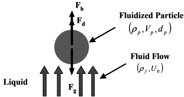
Fig. 1. The balance of forces acting on a fluidized particle in a conventional fluidized bed (liquid media-solid particles).
