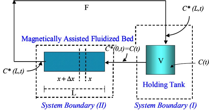
Fig. 3. Schematic diagram of the filtration system.
