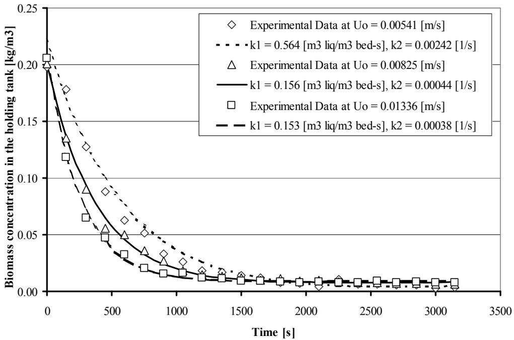
Fig. 6. Change of biomass waste concentration versus flow rate,  $d_p = 3.5$  mm and  $D_p = 180\mu\text{m} < D_p < 295\mu\text{m}$
