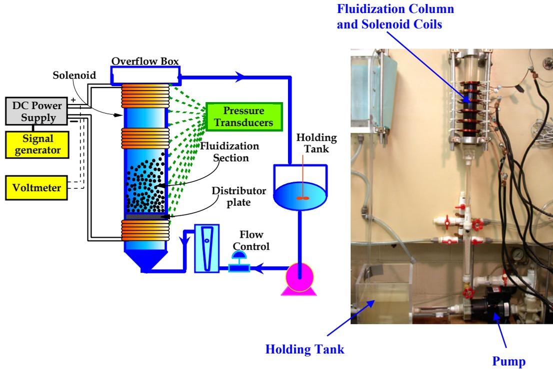
Fig. 4. G-MAFB apparatus used in filtration experiments
