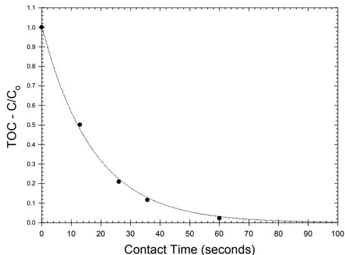
**Figure 7.** Oxidation of 20.7 mg/L of Propylene Glycol (1,2-propanediol) over RP-121 Catalyst Using Oxygen as the Oxidant.
