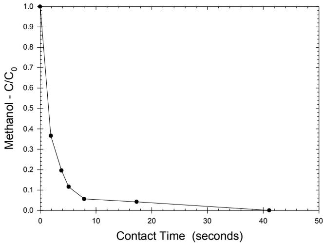
**Figure 3.** Alcohol Oxidase Catalyzed Ambient Temperature Decomposition of 7.9 mg/L Methanol Solution.
