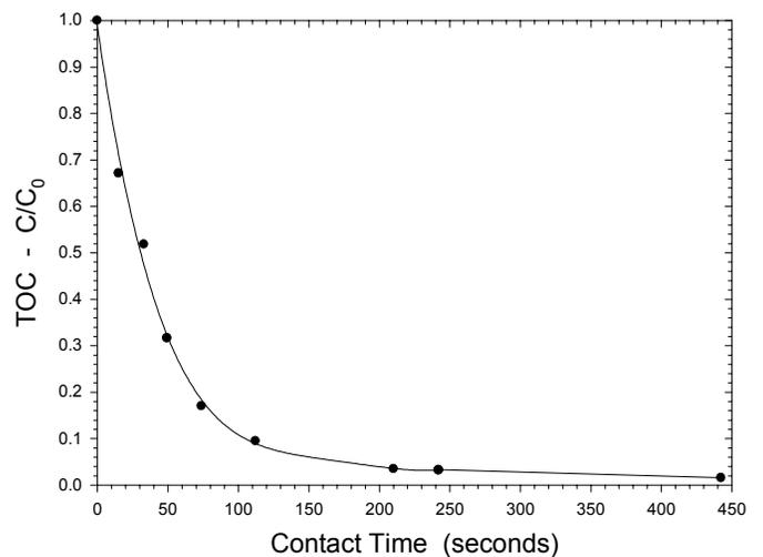
**Figure 5.** Ethylene Glycol Oxidation over RP-121
