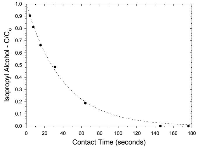
**Figure 4.** Isopropyl Alcohol Oxidation over RP-121
