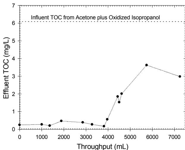
**Figure 10.** Effluent TOC for Integrated System with Acetone Removal by Ambersorb 572.
