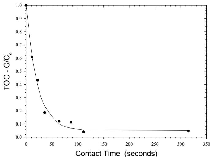
**Figure 6.** Propylene Glycol Oxidation over RP-121
