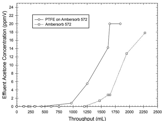
**Figure 8.** Acetone Breakthrough Curves for Uncoated and PTFE Coated Ambersorb 572 Beads.
