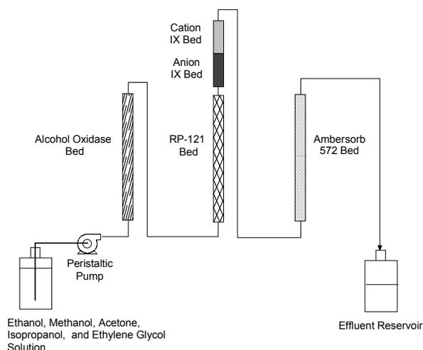
**Figure 9.** Integrated Bioreactor with Acetone Separation by Adsorption.
