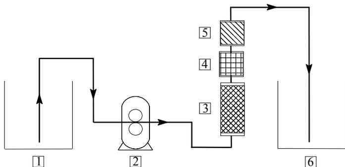
**Figure 1.** Continuous Flow Test Apparatus: 1- Influent Reservoir, 2- Peristaltic Pump, 3- Fixed Enzyme Bed, 4- Fixed Catalyst Bed, 5- Sorbent Bed, 6- Effluent Reservoir.
