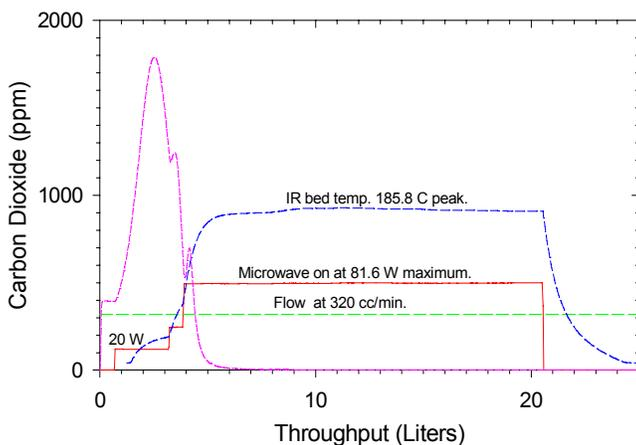
**Figure 5.** Microwave Powered Thermal Regeneration of Carbon Dioxide Loaded Molecular Sieve 5A.
