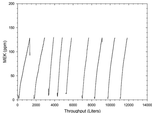
**Figure 14.** Multiple MEK Adsorptions for Activated Carbon Waveguide Cartridge.
