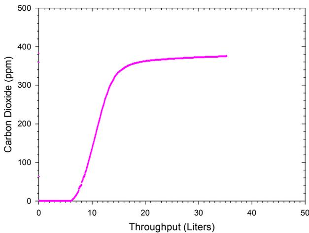
**Figure 4.** Third Sorption of Carbon Dioxide (dry) on Molecular Sieve 5A.
