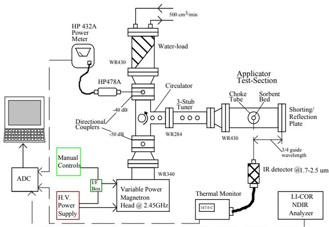
**Figure 1.** Rectangular Waveguide based Microwave Sorption-Desorption Test System.
