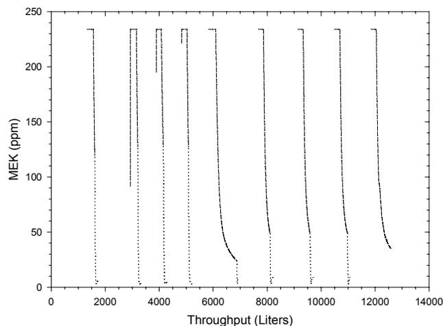
**Figure 15.** Multiple MEK Desorptions for Activated Carbon Waveguide Cartridge.
