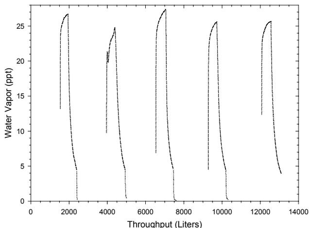
**Figure 13.** Multiple Water Vapor Desorptions for 13X Waveguide Cartridge.
