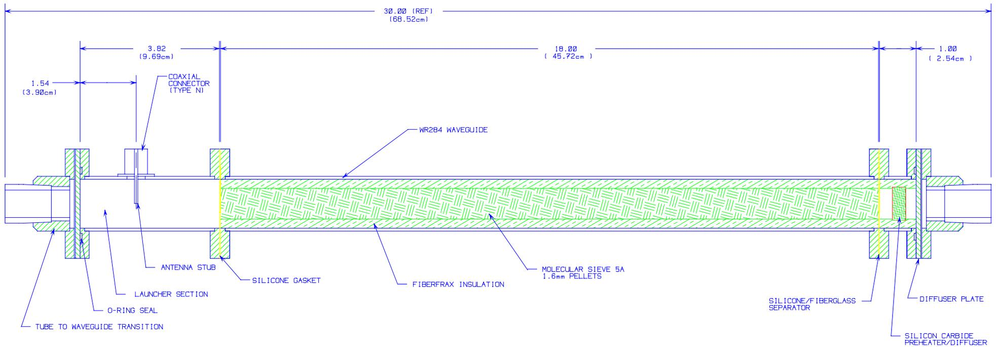
**Figure 6.** Molecular Sieve 5A Waveguide Cartridge.
