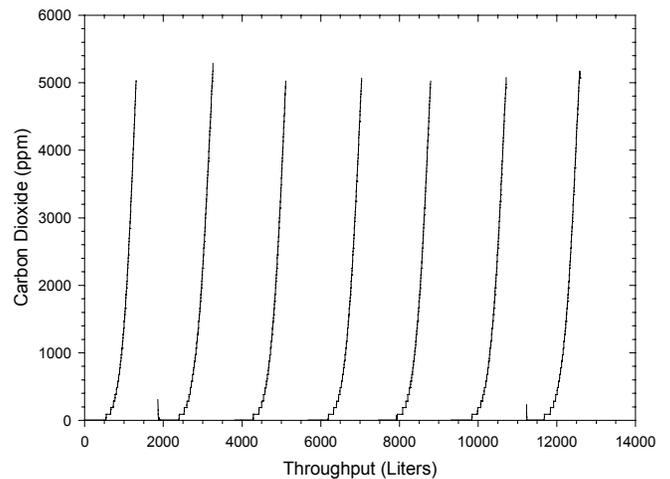
**Figure 10.** Multiple Carbon Dioxide Adsorptions for MS 5A Waveguide Cartridge.
