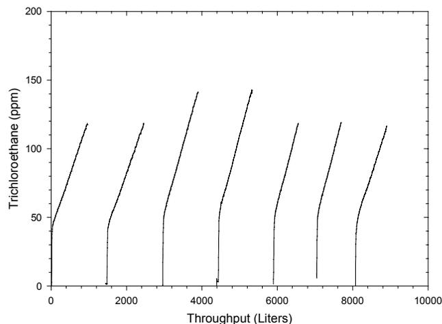
**Figure 18.** Multiple TCA Adsorptions for Activated Carbon Waveguide Cartridge.
