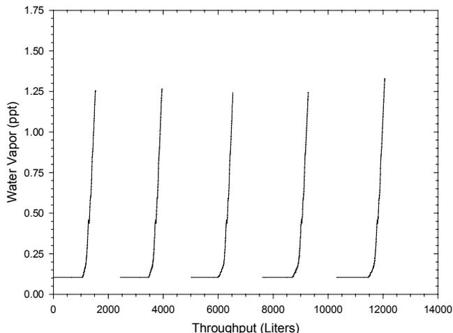
**Figure 12.** Multiple Water Vapor Adsorptions for MS 13X Waveguide Cartridge.
