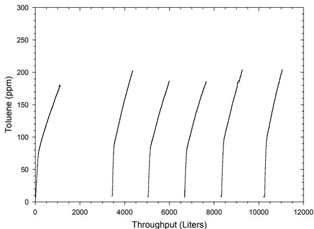
**Figure 16.** Multiple Toluene Adsorptions for Activated Carbon Waveguide Cartridge.
