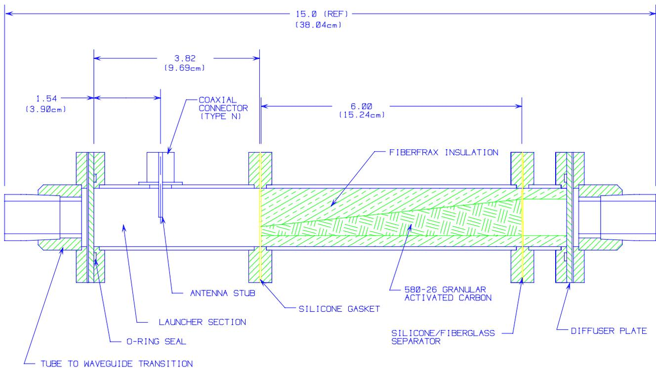
**Figure 8. Activated Carbon Waveguide Cartridge.**
