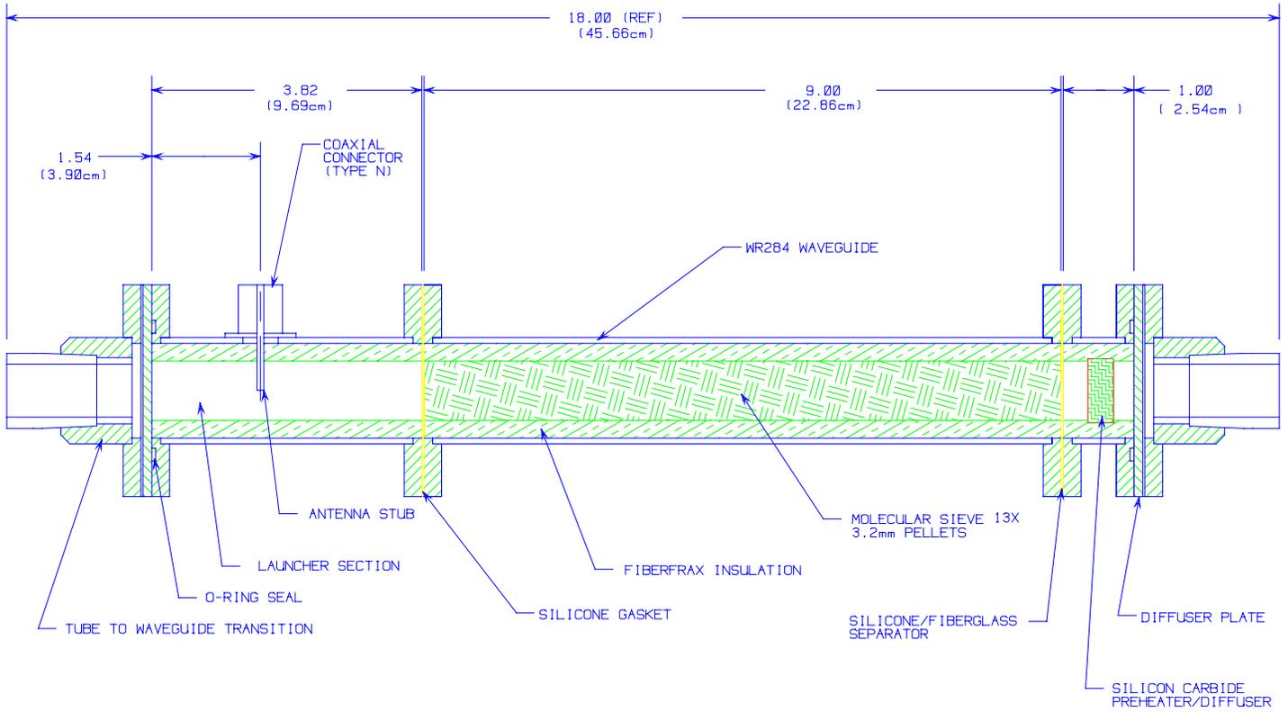
**Figure 7. Molecular Sieve 13x Waveguide Cartridge.**
