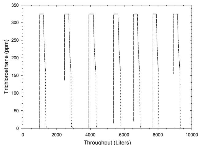
**Figure 19.** Multiple TCA Microwave Desorptions for Activated Carbon Waveguide Cartridge.
