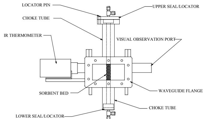
**Figure 2.** Cross Section View of Sorbent Bed Mounted in the Microwave Applicator Section of the Rectangular Waveguide Test System. The direction of Microwave Propagation is orthogonal to the paper. Gas is fed through the fittings located at the bottom and exits at the top.
