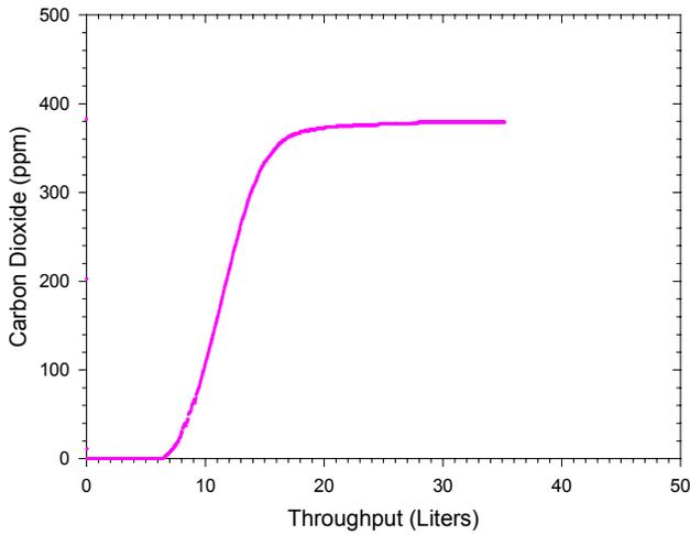
**Figure 3.** Second Sorption of Carbon Dioxide (dry) on Molecular Sieve 5A.
