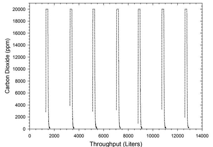
**Figure 11.** Multiple Carbon Dioxide Desorptions for MS 5A Waveguide Cartridge.
