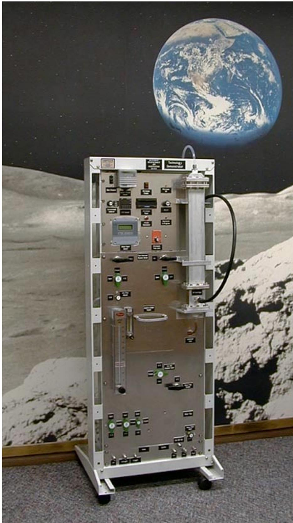
**Figure 20.** Microwave Regenerable Air Purification Technology Demonstrator.
