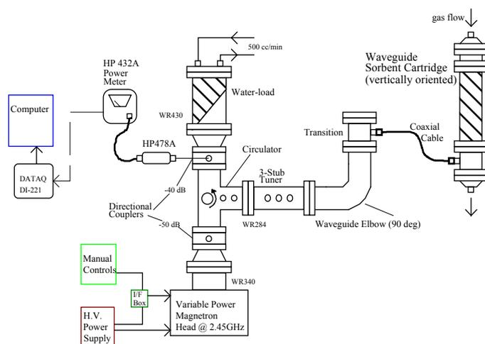
**Figure 9.** Technology Demonstrator Bench-top Testing Microwave Power Diagram.
