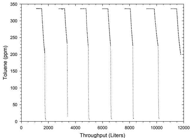
**Figure 17.** Multiple Toluene Desorptions for Activated Carbon Waveguide Cartridge.
