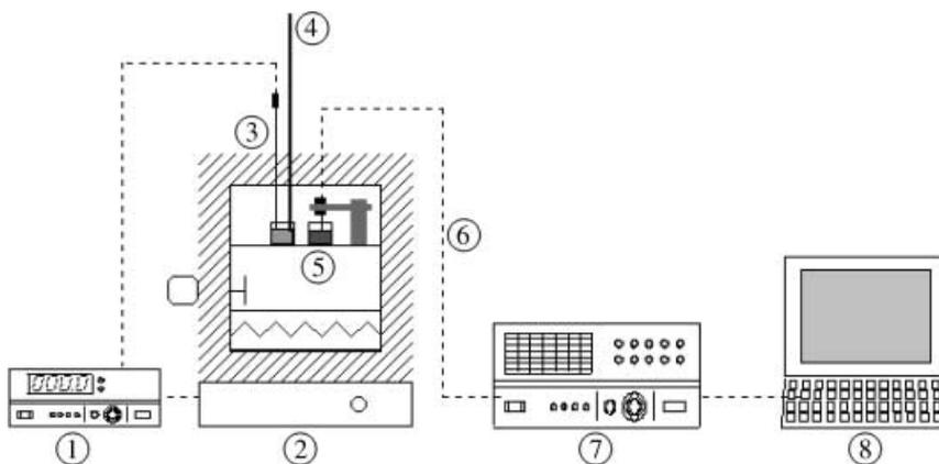
**FIGURE 2** Complex permittivity test apparatus: (1) temperature controller, (2) oven, (3) thermocouple, (4) Hg thermometer, (5) dielectric probe immersed in sample, (6) high-temperature semi-rigid coaxial cable, (7) vector network analyzer, and (8) computer
