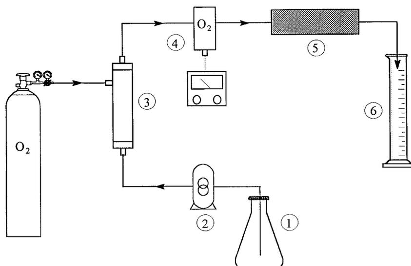
Fig. 1. Oxygen saturation subsystem. (1) D-glucose solution, (2) peristaltic pump, (3) membrane oxygen saturator, (4) in-line dissolved oxygen electrode and meter, (5) immobilized glucose oxidase bed, (6) sample collection vessel.
