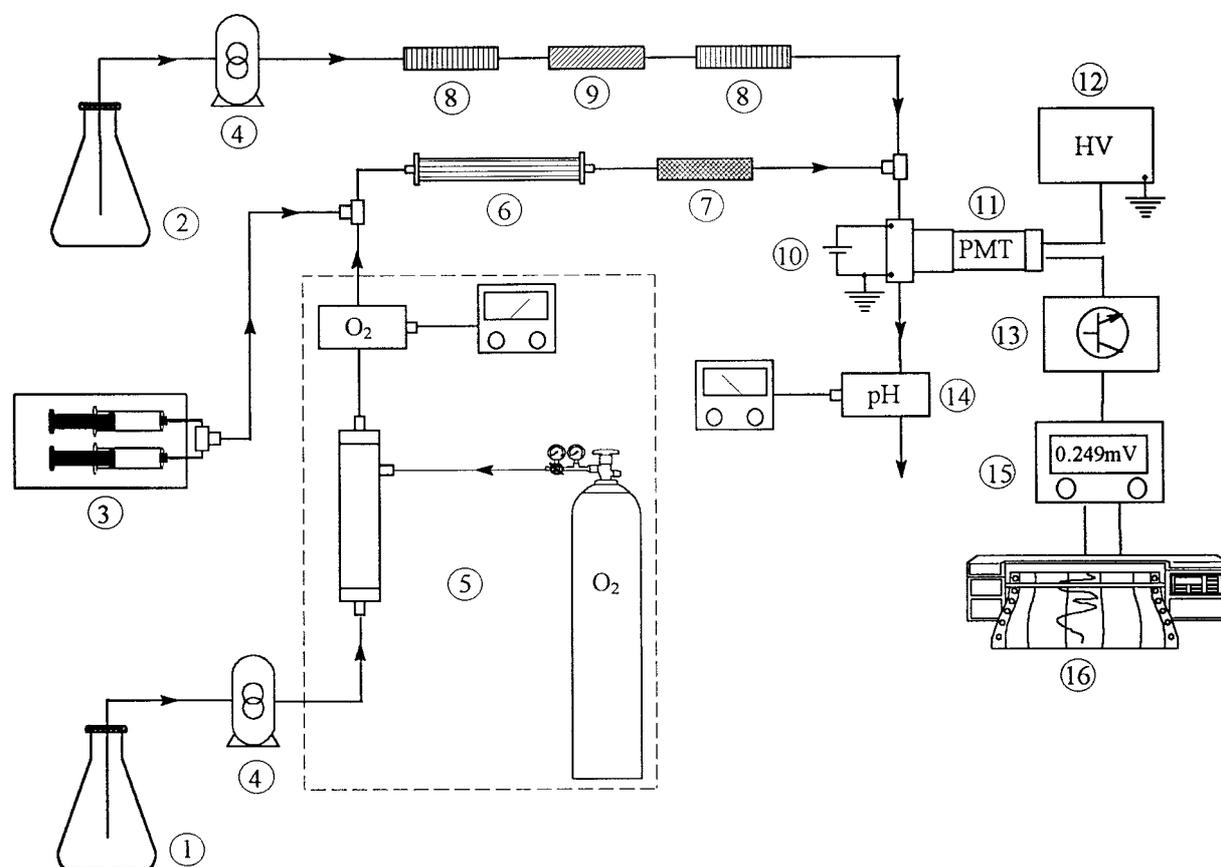
Fig. 2. Reagentless glucose and  $O_2$  chemiluminescence experimental apparatus: (1) D-glucose solution ( $O_2$  detection mode), DI water (glucose detection mode), (2) DI water, (3) syringe pump, (4) peristaltic pump, (5)  $O_2$  saturation subsystem, (6) ultrafiltration membrane, (7) glucose oxidase bed, (8) SPB, (9) SPL, (10) ECL observation cell, (11) PMT, (12) power supply, (13) signal conditioning, (14) pH probe, (15) digital voltmeter, (16) recorder.
