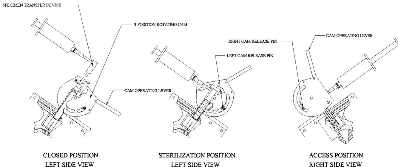
Figure 3. Prototype microwave sterilizable access port.
