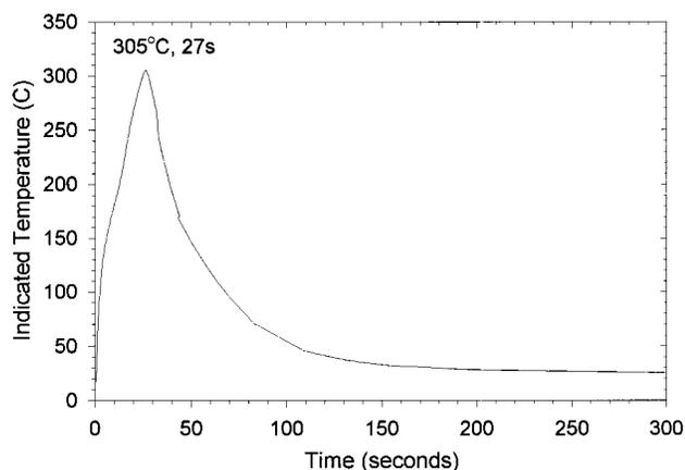
Figure 4. MSAP sterilization chamber temperature profile.
