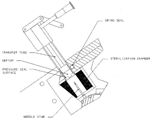
**Figure 2.** Materials transfer interface mated with the miniaturized sterilization chamber. Prior to accessing the microbially vulnerable system, the exposed surface of the septum and the needle stub are sterilized. Following sterilization, the rotating cam forces the needle to penetrate the septum, and aseptic access to the system is achieved.
