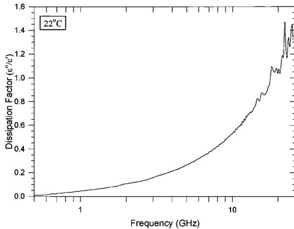
**Figure 6.** Dissipation factor versus frequency for pure water at 22 °C.
