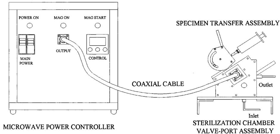
**Figure 1.** Components of the prototype microwave sterilizable access port.
