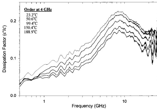
**Figure 5.** Dissipation factor versus frequency for  $\alpha$ -SiC between 23 and 189 °C.
