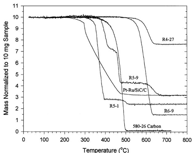
Fig. 14. TGA results from ambient temperature to 800°C at 10°C/min.
