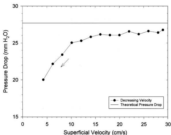
Fig. 2. Minimum fluidization velocity of activated carbon at 1350°C.
