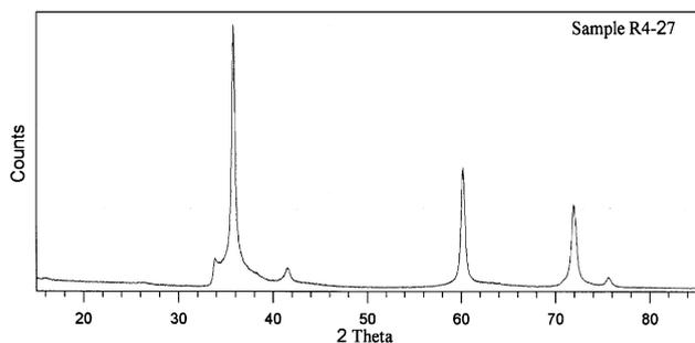
Fig. 3. X-ray diffractogram for silicon-carbide-coated activated carbon sample R4-27. 5 h reaction time at 1350°C with introduction of 1 g SiO at 30 minute intervals.
