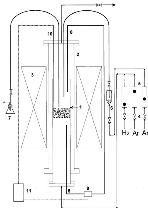
Fig. 1. High-temperature fluidized bed reactor (HTFBR) schematic: 1, fluidized-bed reactor; 2, furnace tube; 3, furnace; 4, control valve; 5, flowmeter; 6, pneumatic solid charger; 7, pneumatic solid discharger; 8, pressure probe; 9, pressure transducer; 10, thermocouple; 11, data acquisition system.
