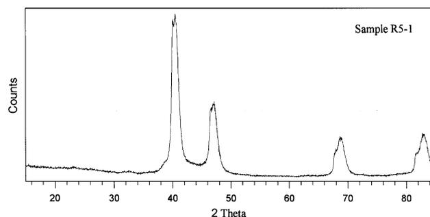
Fig. 6. X-ray diffractogram for RP-121 catalyst treated at 1350°C for 1 h.
