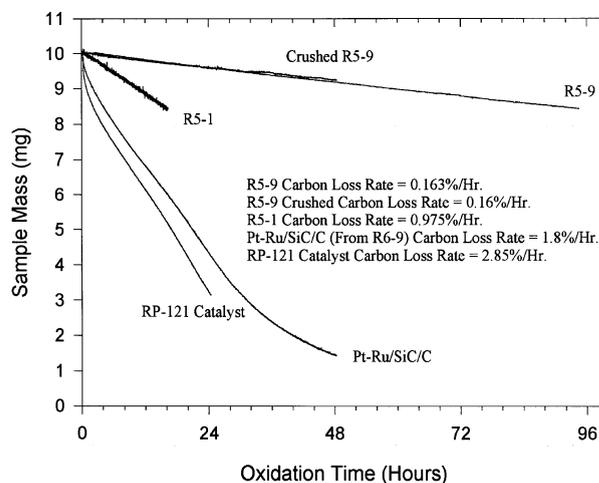
Fig. 16. Isothermal TGA of catalysts at 245°C.
