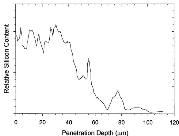
Fig. 12. Silicon distribution in cross-section of a silicon-carbide-coated carbon granule.
