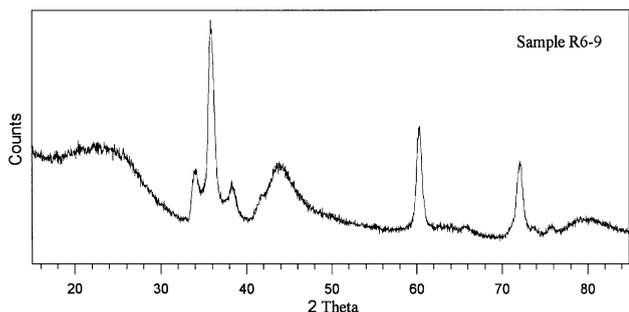
Fig. 4. X-ray diffractogram for silicon-carbide-coated activated carbon: sample R6-9. 8 h reaction time with the introduction of 0.5 g SiO at 30 minute intervals.
