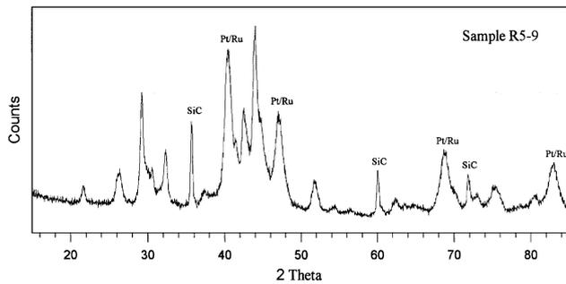
Fig. 7. X-ray diffractogram for SiC-coated RP-121 catalyst. Treated at 1350°C for 8 h with 0.5 g SiO introduction at 30 minute intervals.
