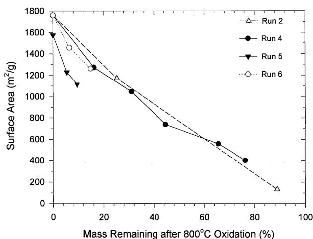
Fig. 17. BET surface area versus oxidation resistance resulting from SiC formation.
