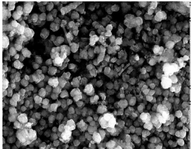
Fig. 9. Scanning electron micrograph of SiC/C — sample R2-20 (8500×).
