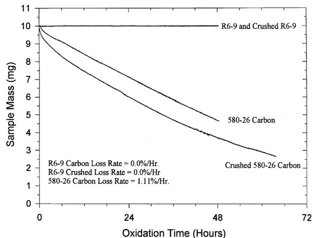
Fig. 15. Isothermal TGA of SiC/C and 580-26 activated carbon substrate at 245°C.
