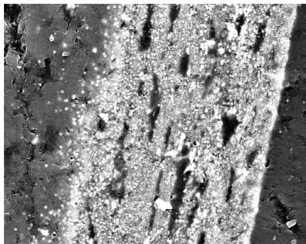
Fig. 13. Scanning electron micrograph of  $\text{SiC}$  to  $\text{C}$  transition (1700 $\times$ ).
