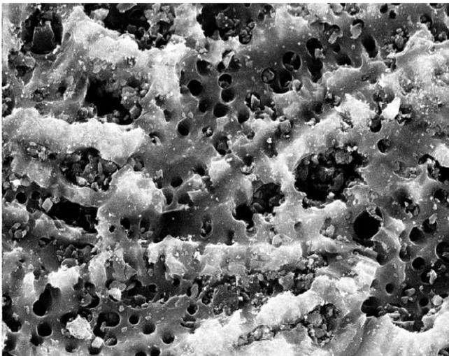
Fig. 8. Scanning electron micrograph — untreated 580-26 activated carbon (2000×).
