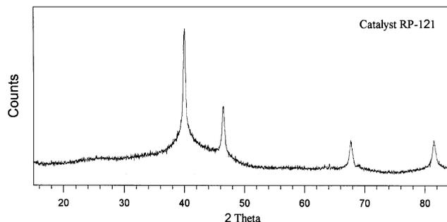
Fig. 5. X-ray diffractogram for untreated RP-121 carbon-supported catalyst.
