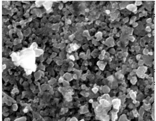
Fig. 10. Scanning electron micrograph of SiC/C — sample R4-27 (20,000×).
