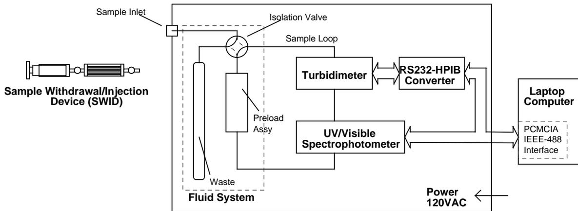
**Figure 3, Spectrophotometer System Schematic, Illustrating the Sampler (SWID), Fluid Loop, and Communication Bus to an External Laptop Computer**
