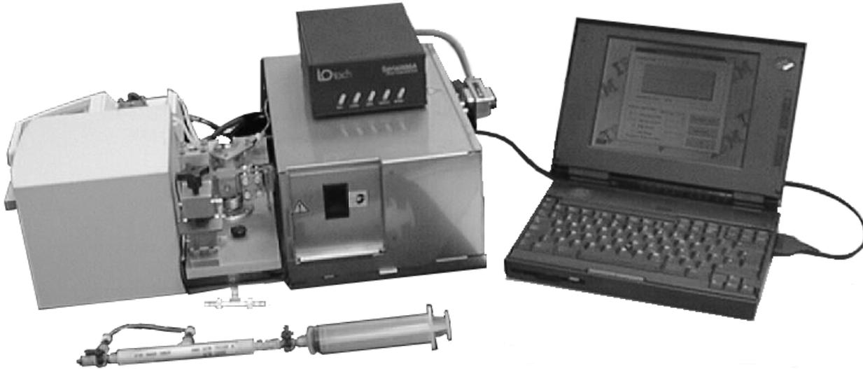
**Figure 1, Prototype Spectrophotometric Analyzer, Consisting of a HP8453a Ultraviolet-Visible-NearIR Spectrophotometer and a Hach 2100P Ratio Turbidimeter.** A sample syringe and membrane-based deaerator are shown in front of the instrument, next to a control processor (laptop computer) that operates the instrument via an IEEE 488 interface.
