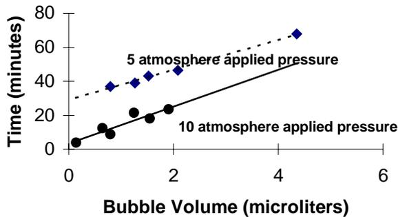
**Figure 5, Single Bubble Dissolution Times in 5 Milliliter Sample Volumes as a Function of Time, Bubble Volume, and Applied Pressure.**
