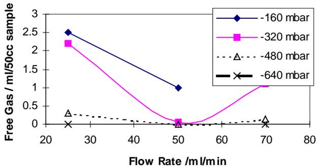
**Figure 4, Residual Free Gas vs. Flow Rate and Applied Vacuum**
