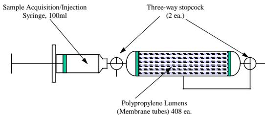
**Figure 2, Sample Withdrawal/Injection Device (SWID), a Two-Pass Flow-Through Membrane Deaerator.**
