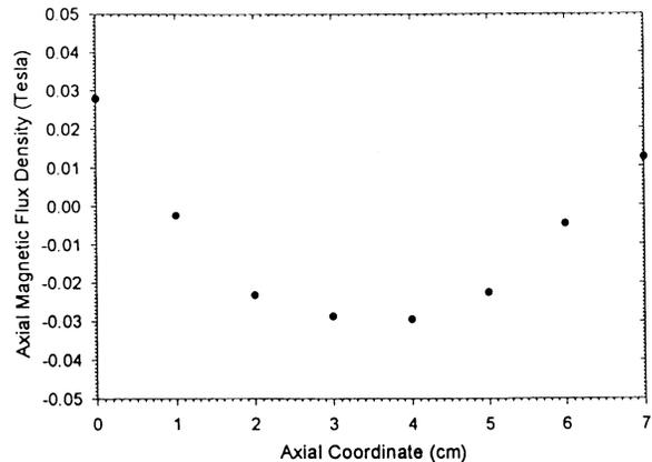
Figure 14. Axial Magnetic Flux Density for the 7 cm Ring Spacing.
