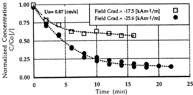
Figure 12. Filtration with and without Magnetic Consolidation of Granular Media.
