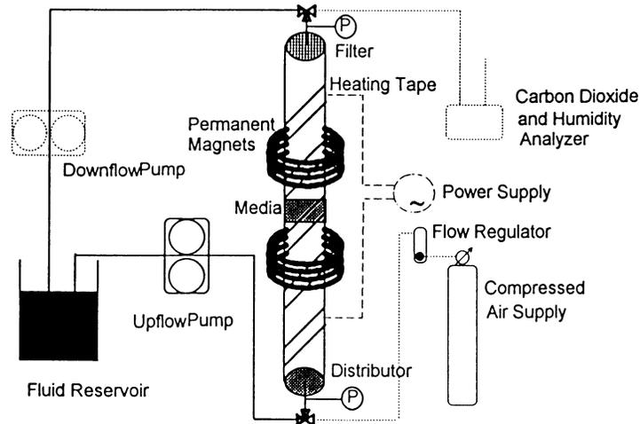
Figure 15. Permanent Magnet based MSFB Test Stand
