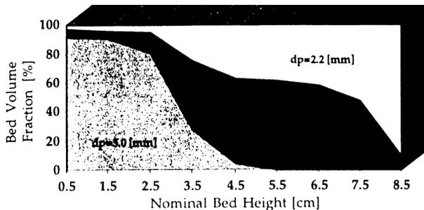
Figure 10. Particle Stratification by Magnetic Field Gradient ( $-21.5$   $\text{kAm}^{-1}/\text{m}$ ).
