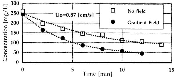
Figure 11. Particle Stratification by Magnetic Field Gradient (-21.5 [kAm<sup>-1</sup>/m]).
