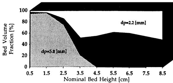
Figure 9. Particle Distribution in Bed without Magnetic Field.
