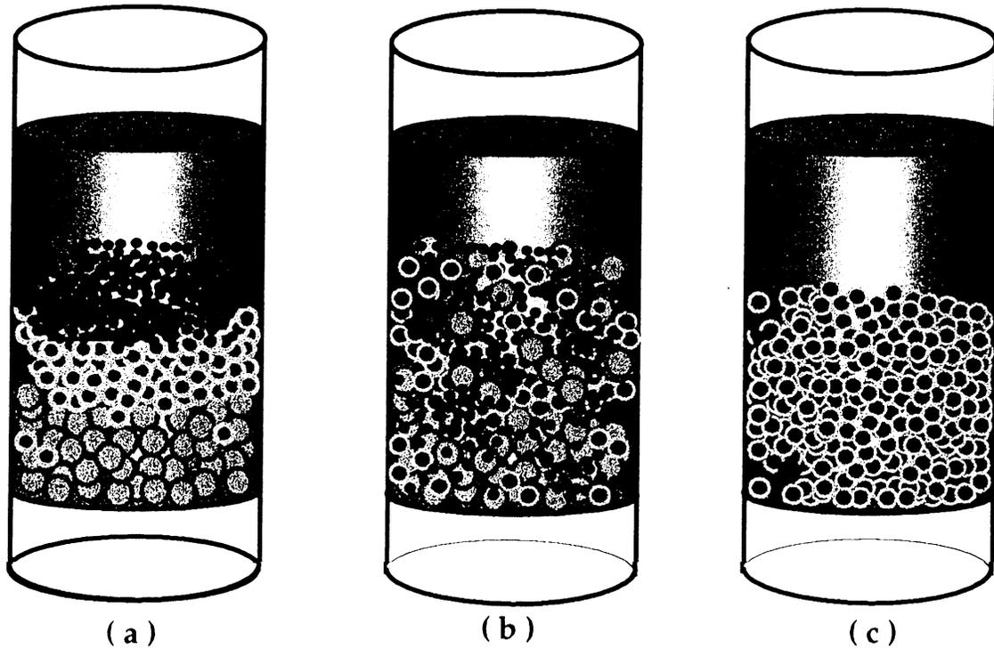
Figure 8. Three Different Types of Filter Media Packing: a) Stratified, b) Random, c) Monosize.
