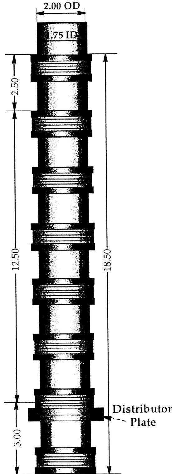
Figure 7. Schematic of a CGMSFB system with Eight Helmholtz Rings.
