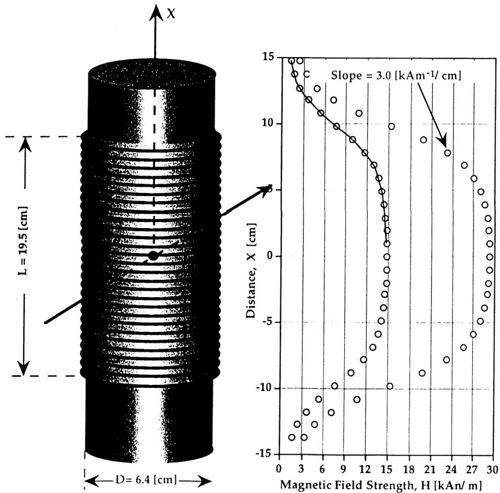
Figure 5. Field strength along the central axis of CCMSFB.
