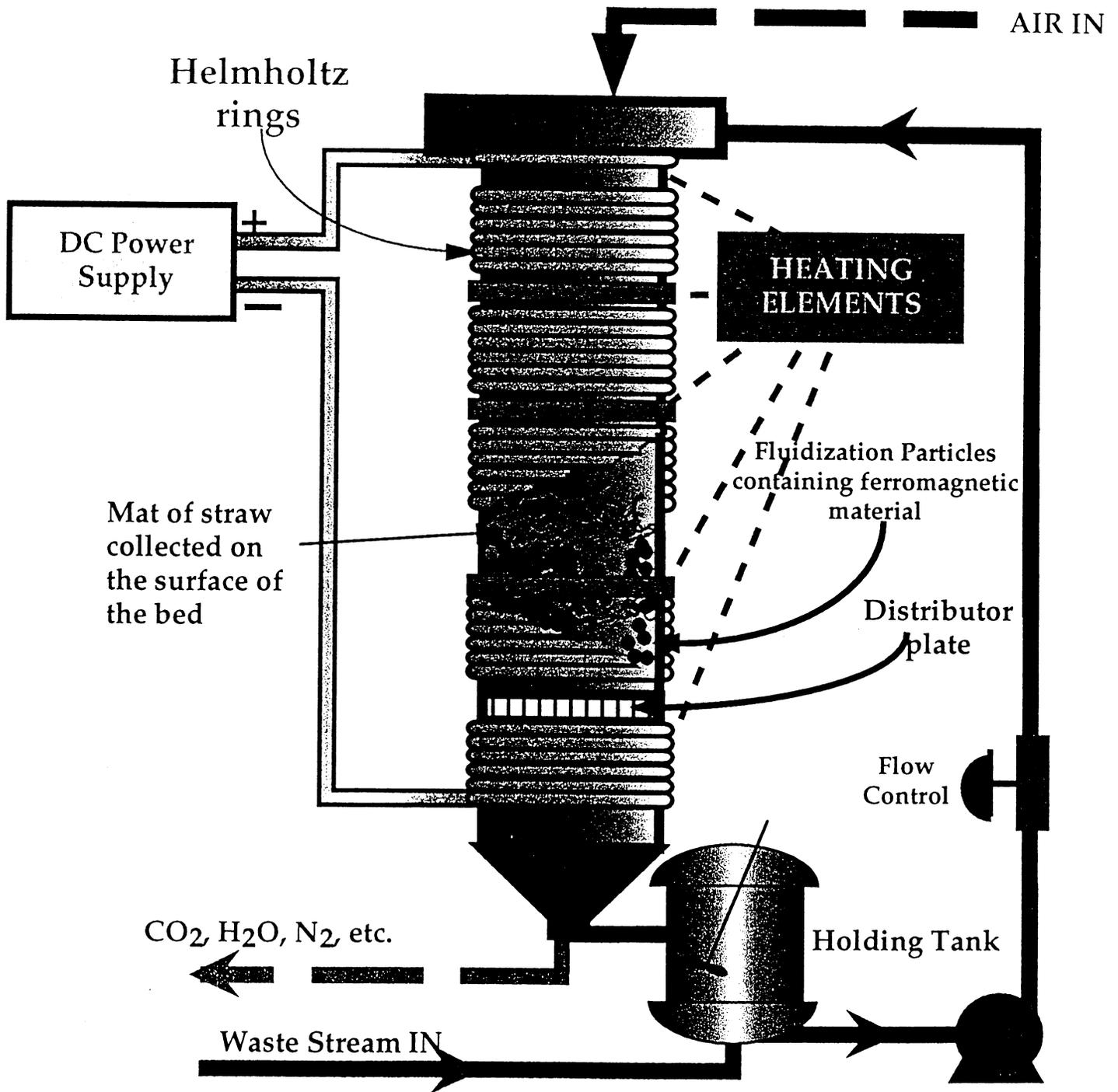
Figure 1. Three Step Magnetically Assisted Solid Waste Destruction Process
