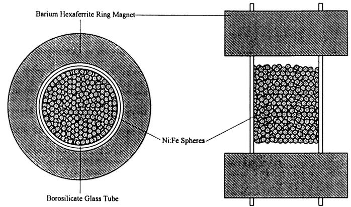
Figure 13. Ring Magnet Configuration for Gravity Independent Confinement.
