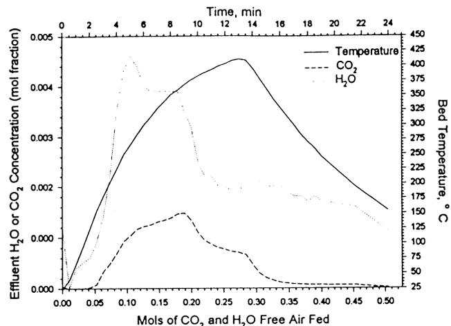
Figure 16. Combustion of Inedible Plant Biomass in Integrated Test.
