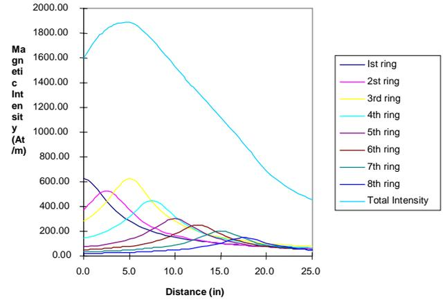
Figure 4. Axial Field Intensity for System of Eight Helmholtz Coils.
