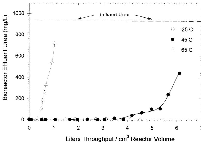
Figure 4. Urease Bioreactor Performance Between 25°C - 65°C for 1000 mg-L<sup>-1</sup> Urea Influent.
