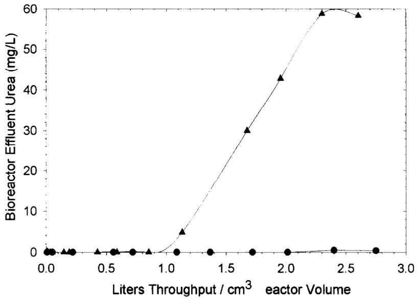
Figure 1. Bioreactor Effluent Urea Levels for 60 mg-L<sup>-1</sup> Influent: with 0.8 mg-L<sup>-1</sup> Dissolved Elemental Iodine (triangle), and without Iodine (circle).
