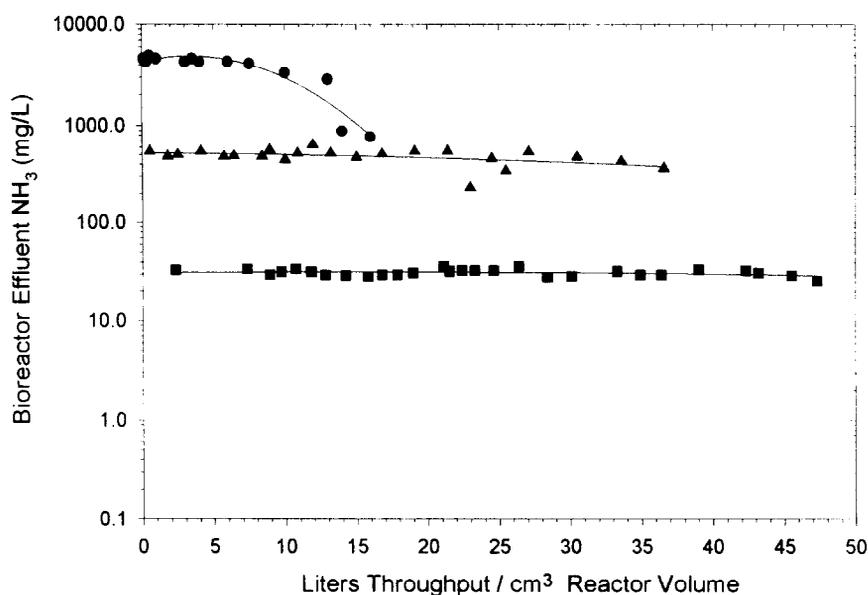
Figure 3. Bioreactor Effluent Ammonia Levels for 60 mg-L<sup>-1</sup> (square), 1000 mg-L<sup>-1</sup> (triangle), and 10000 mg-L<sup>-1</sup> (circle) Influent Urea Concentrations.
