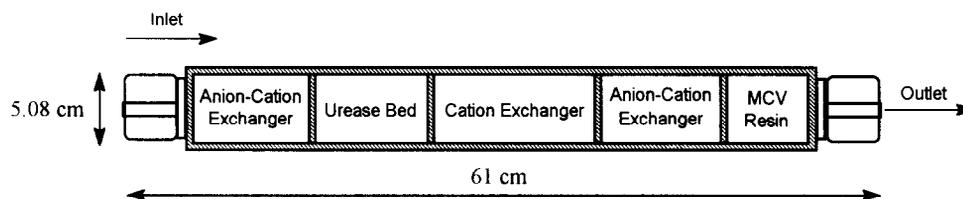
Figure 5. Full Scale Breadboard Urease Bioreactor - Layered Sorbent Module.
