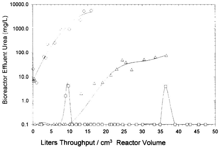
Figure 2. Bioreactor Effluent Urea Levels for 60 mg-L<sup>-1</sup> (square), 1000 mg-L<sup>-1</sup> (triangle), and 10000 mg-L<sup>-1</sup> (circle) Influent Urea Concentrations.
